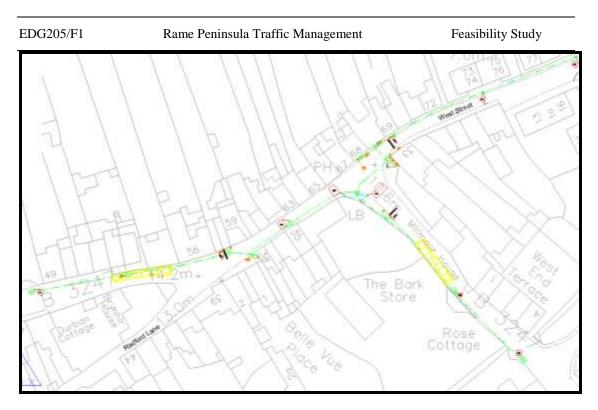
Figure 9.3: Extract from Drawing EDG\_0205\_07 Diagrammatic plan for three-way traffic signals
